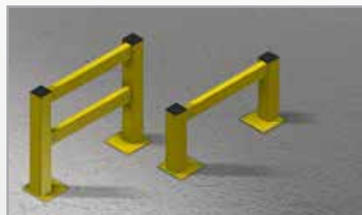
C-Rail Barriers - Designed to protect end of racks as well as pedestrian walkways and made from 5mm thick material to offer sturdy protection. (Options available - Width: 460mm or 760mm Depth options: • 900 • 1100 • 2000 • 2400)
